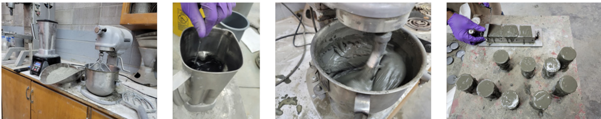
Figure 2: Graphene-cement mixture preparation from left to right are: High shear rate mixer and Hobart bowl; aqueous dispersed graphene solution; graphene-cement paste in Hobart mixer; cube and cylinder molds with graphene-cement paste.
